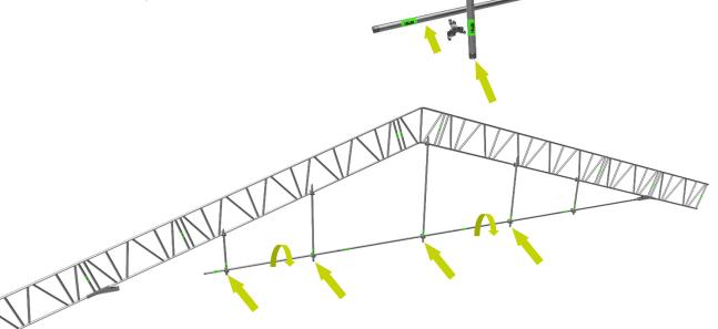
Continue as detailed adding further lengths of tubelok as required. Droppers to be added progressively to keep tube locked at maximum 3.0m c/c or as specified by designer.
