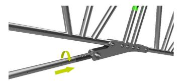
Connect first length of TubeLok and rotate to lock in position and align coupler mark.
