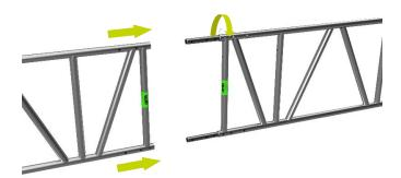
Insert and secure Pins as shown for top joint Connect next lattice beam
