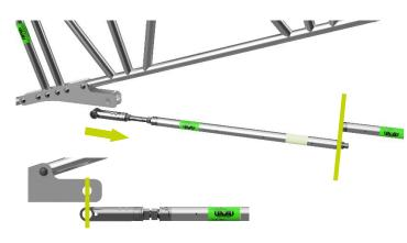
Slide Assembly between the pins of the Tension Bar End Plate Assembly past the 32mm hole
