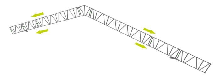
Rotate Tension Bar End Plate Assembly insert the remaining of the M12 Bolts Washers and Nuts.
